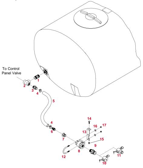
NOTE: Apply thread sealant to the fittings. Do not use sealant on external threads of tank outlet fitting.
